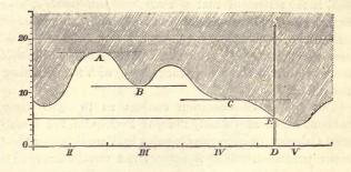
To find then what was the temperature at any instant, say  $4^{h}.41^{m}$ , all we have to do is to draw (as in the figure) the line DE which at that time must have coincided with the slit. The point E, where this line meets the boundary of the blackened part of the paper, indicates where the end of the mercury column was at the given instant. In the figure, as drawn, the temperature is  $5^{\circ}.2$ .
